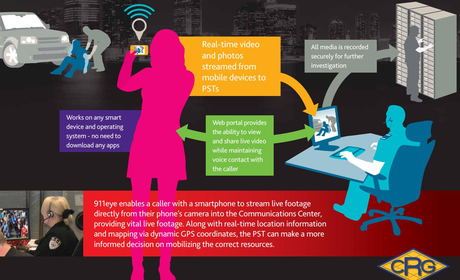
911eye enables a caller with a smartphone to stream live footage directly from their phone's camera into the Communications Center, providing vital live footage. Along with real-time location information and mapping via dynamic GPS coordinates, the PST can make a more informed decision on mobilizing the correct resources.
